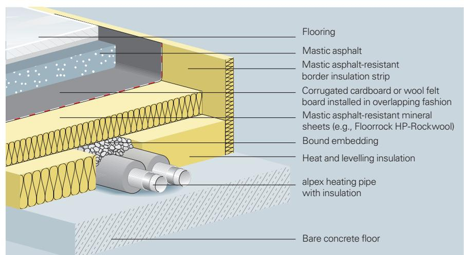
Floor structure under mastic asphalt
