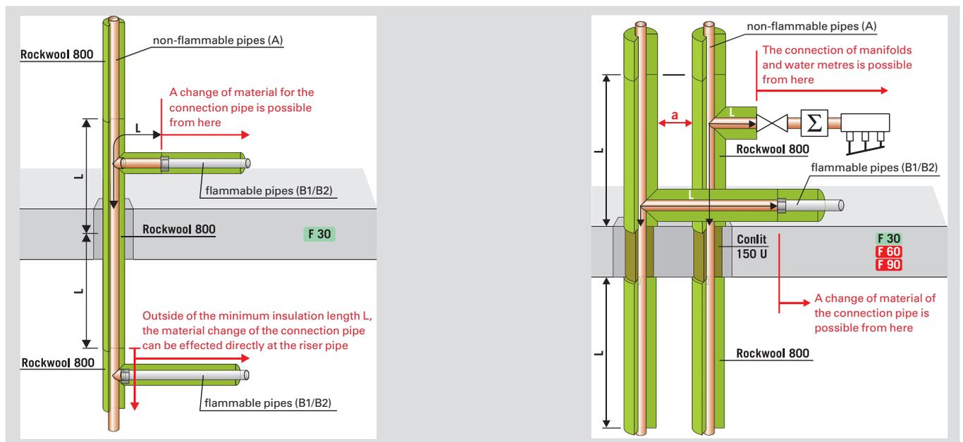
Connection pipes in riser pipes with feed-through insulation R 30, maintaining a minimum insulation length L on both sides of the feed-through ( $L \geq 500$  mm).
