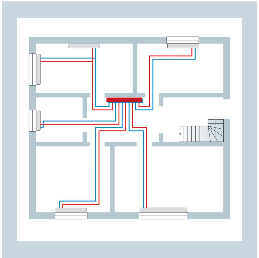
Floor plan with heating circuit routing
