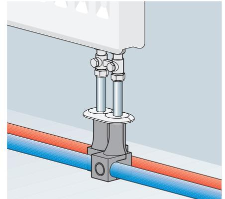
alpeX loop pipe with radiator connection tee
