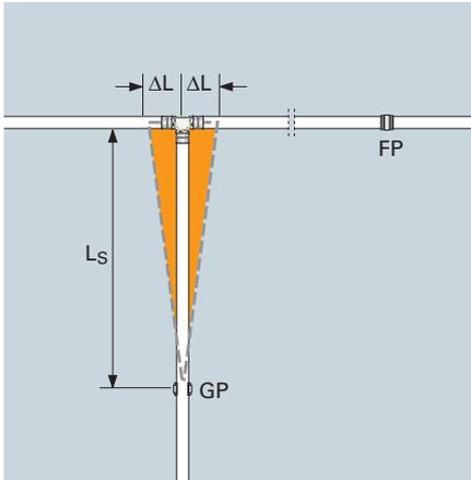
Compensation for length change with an expansion bend "L<sub>s</sub>"
