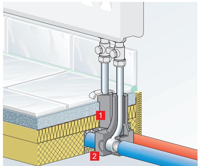
The isolation of the crossover tee is achieved by the noise absorption kit. This involves embedding of the metal body of the crossover tee into the two-part noise absorption kit.
