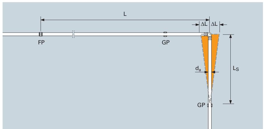
Compensation for length change using an expansion bend "L<sub>s</sub>"
