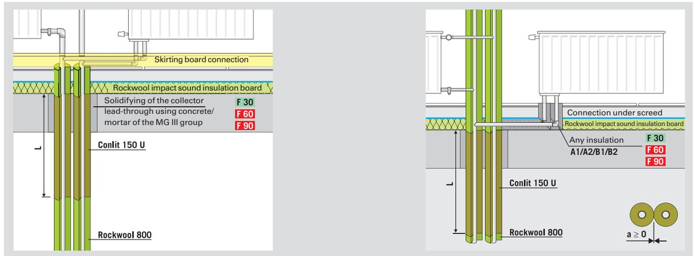
R 30 to R 90 fire stops for radiator connection pipes of metal composite pipe  $d \leq 63$  mm, maintaining a minimum insulation length L on one side of the feed-through ( $L \geq 1,000$  mm).
