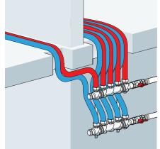
Mounting of the manifold beneath the basement floor
