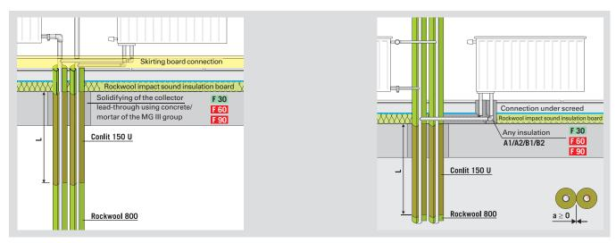
R 30 to R 90 fire stops for radiator connection pipes of metal composite pipe d  $\leq$  63 mm, maintaining a minimum insulation length L on one side of the feed-through (L  $\geq$  1,000 mm).
