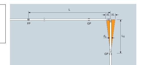
Compensation for length change using an expansion bend  $``\mathsf{L}_{s}''$
