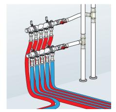
Mounting of the manifold to the building structure
