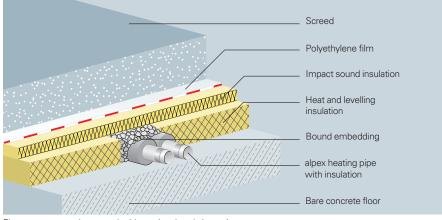
Floor structure under screed with pre-insulated alpex pipe
