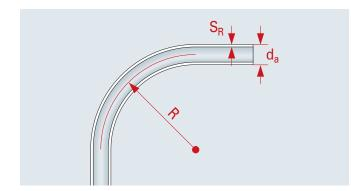
The minimum bend radii R (see figure on the left and table below) must be complied with. alpex connectors must not be used for pipe bending and must only be installed on the finished pipe bend.
