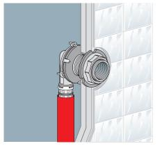
alpex wall feed-through in light-weight construction
