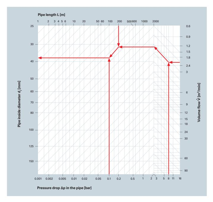
**Example:** The selected nominal diameter of the pipe is DN 40  $\triangleq$  50×4
