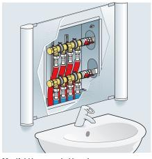
Manifold in concealed housing Manifold located behind a mirror. In this case, the manifold is easily accessible, which is particularly important for decentralised metering.
