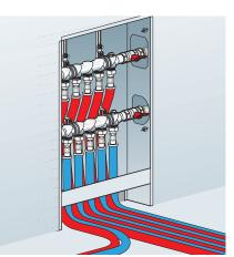
Mounting of the manifold in the manifold cabinet
