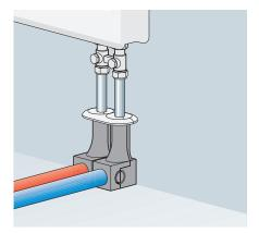
alpex single connection from manifold with radiator connection bend
