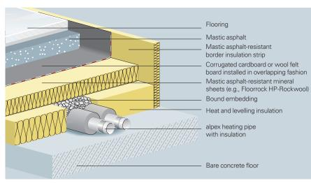
Floor structure under mastic asphalt
