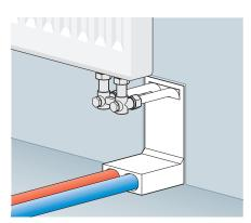
alpex single connection from manifold with radiator connection block
