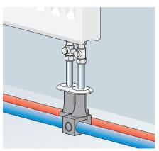
alpex loop pipe with radiator connection tee
