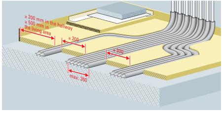
Pipe run widths and supporting area widths
