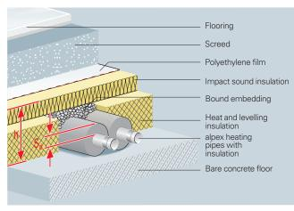
Floor structure with pipe insulation
