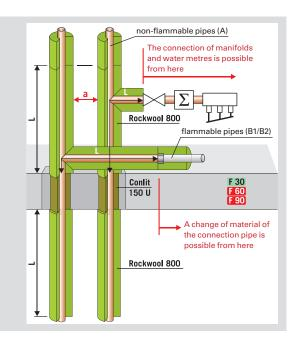
Connection pipes in riser pipes with feed-through insulation R 30, maintaining a minimum insulation length L on both sides of the feed-through (L  $\ge$  500 mm).
