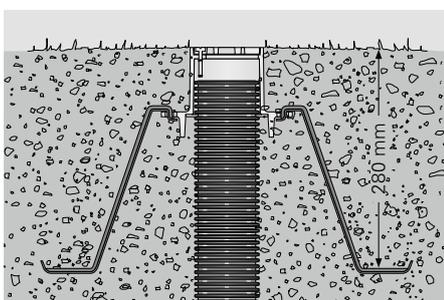
The Walu end cap serves as universal cover element for all surfaces. The retractable and lockable cover allows
