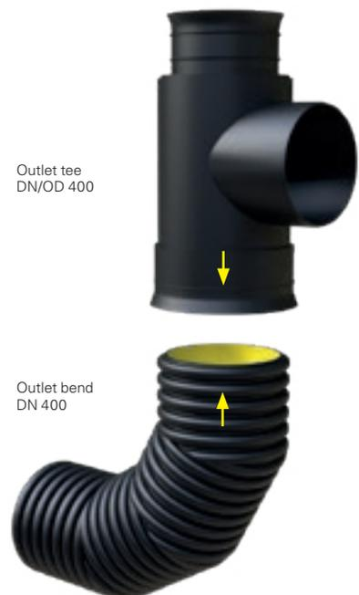
Mount the profile sealing ring DN 400 onto the second corrugation trough of the outlet bend while still outside the excavation pit. Keep the pipe, profile sealing ring, and the coupling clean. Then apply a sufficient amount of lubricant to the profile sealing ring and coupling. Make sure that the sealing area is free of dirt. Connect the outlet bend with the target segment as shown.
