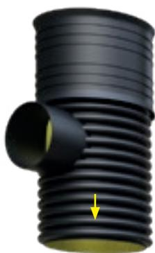
Keep the end of the inlet, the profile sealing ring and the coupling clean. Mount the profile sealing ring onto the second corrugation trough. Then apply a sufficient amount of lubricant to the profile sealing ring and coupling. Make sure that the sealing area is free of dirt.
