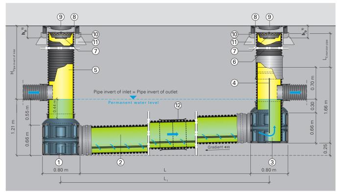
SediPipe level 600/12 with discharge into a surface waterbody or sewer  $^{\eta}$  Adjustable, depending on shaft cover, height, and number of support rings
