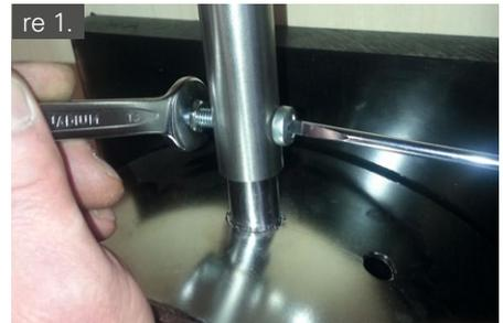
2. We recommend illuminating the bottom of the shaft using an explosion-protected illuminant. Now check whether the stainless steel channel in the shaft is free of contamination; if not, clean/hose it down with water (hose or watering can).
