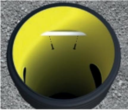
Position the fixture for the lifting bar vertically and centrally over the stainless steel base plate and screw directly into the shaft wall, no primary drilling required.
