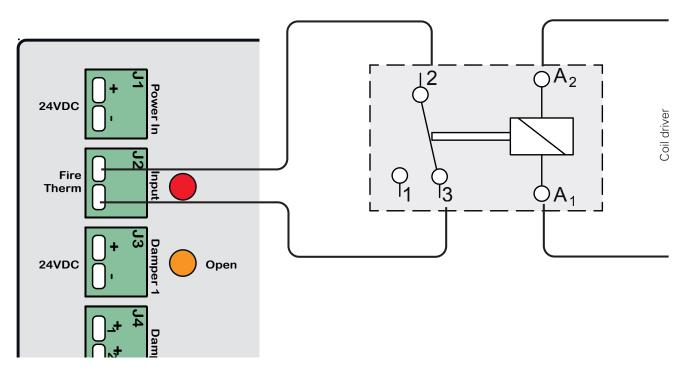
To use the function, the contact must be connected to the break-contact relay (see illustration), and the factory-provided bridge must be removed. If the relay is in a "live" state, the contact is closed. If the current at the relay drops, the contact will be broken and the ventilation unit will be deactivated. The J2 contact is operated at a maximum of 24 V DC/300 mA.
