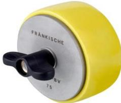
Kabu-BV is an end plug made of a solid rubber core (EPDM) with a soft thermoset elastomer (PUR) jacket in yellow and stainless steel compressive flanges.
