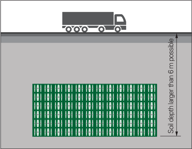
High installation depth of a multiple-layer storage/infiltration system
