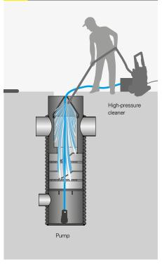
SediPoint's compact design makes cleaning the complete shaft very easy. The cleaning does not require companies providing sewer flushing. After removing the operating pipe, the mud is easily vacuumed from the mud chamber. Mobile wastewater pumps or cleaning/vacuum trucks are suited for this.
