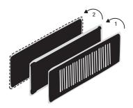
The innovative clamp and sealing connection ensures a secure fit of the design grill in the mounting frame.
